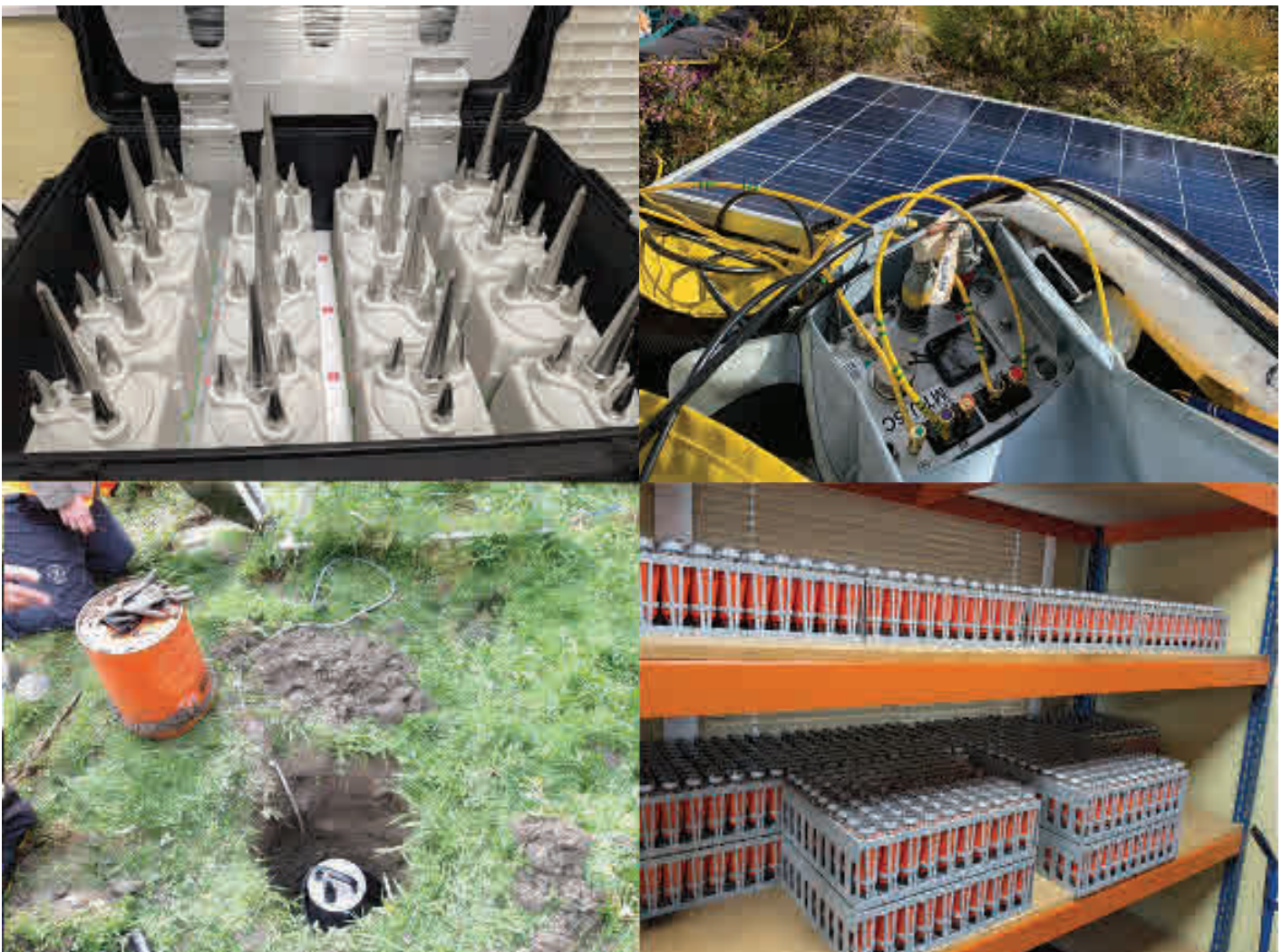
1 Top left: SmartSolo node battery packs under charge; Bottom left: A broadband seismometer being deployed, ready to be covered then buried; Bottom right: A subset of the 1980 Stryde nodes at the LeNS-UK facility; Top right: Phoenix MTU-5C ultra-wideband magnetotelluric receiver close to Coire an t-Sneachda. (Nick Rawlinson, Juliane Hübert, Jack Andrew Smith, University of Edinburgh)
